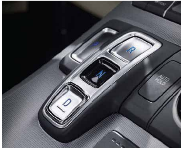
8-speed shift-by-wire automatic transmission
